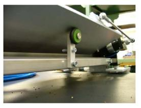
The seed tray can be tilted upwards as shown when sowing smaller seeds or smaller quantities. Loosen the fixing screw and adjust the roller arm to suit.
