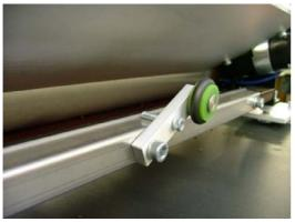
The normal running position for the rear roller is shown here.
