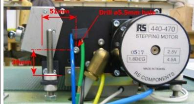
7) Fit the short spring post to the datum end plate using the hole drilled in step 5.
