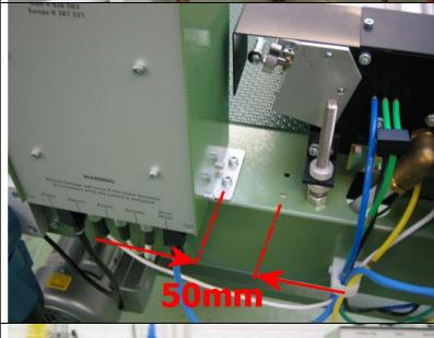
5) Drill a 5.5mm diameter hole in the datum end plate as shown. Dimensions are measured from the edges of the datum end plate. (51mm and 39mm)
