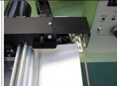
14) Fit the switch to the control box – we suggest the position shown – from where the air jet flow control was removed.
