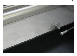
Remove the ball joint where it connects to the tray..
