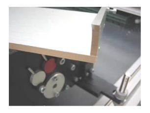
Carefully inspect the fabric covered edges of the seed tray for signs of damage. Under no circumstances use the tray if the fabric is missing or damaged, as it may cause irreparable damage to the drum. Wash the seed tray using warm, soapy water and a soft cloth. Do not use solvents of any kind, as they can remove the adhesive backing of the fabric.
