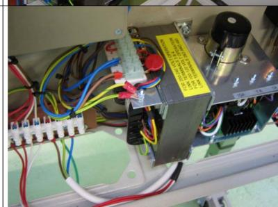
17) Wire the output from the transformer to the motor, connecting the positive wire via the switch.
