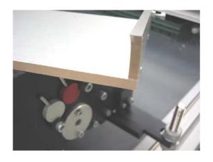
Carefully inspect the fabric covered edges of the seed tray for signs of damage. Under no circumstances use the tray if the fabric is missing or damaged, as it may cause irreparable damage to the drum. Wash the seed tray using warm, soapy water and a soft cloth. Do not use solvents of any kind, as they can remove the adhesive backing of the fabric.
