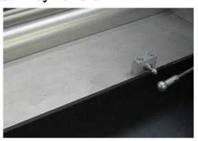
Remove the ball joint where it connects to the tray..
