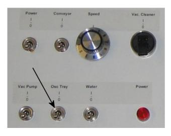
Turn on the seeder power switch on the top of the main control box, and then the Osc. Tray switch. The tray will run until the switch is turned off, or the main power is turned off. Avoid running the tray for long periods without sowing, to preserve the life of the anti-wear impregnated fabric material.
