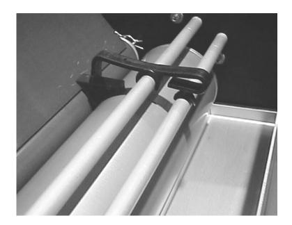
The Seed Valley End Seals replace the original Drum 'V' Brushes, which had a tendency to splay out and become ineffective if not maintained correctly. The plastic seals are manufactured from hard-wearing high-impact ABS material and should last for several seasons if used in accordance with the instructions.
