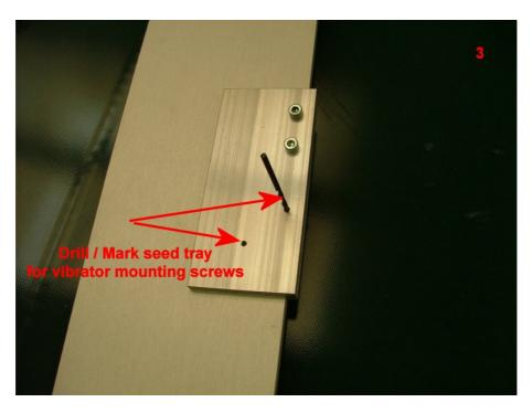
3) Using the 3.5mm drill provided, drill through the template and tray to provide a pilot hole
