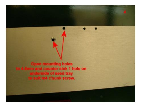
4) Turn the tray over, and drill through the pilot holes to open them out with a 4.5mm drill. Countersink the lower hole so that the head of the countersunk screw will be flush with the surface.
