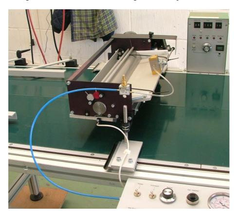
It is necessary to drill two holes in the tray base to attach the vibrator. The position of these holes is important, and your distributor can provide a jig to ensure accurate positioning. Please ensure the jig is returned after fitting.
